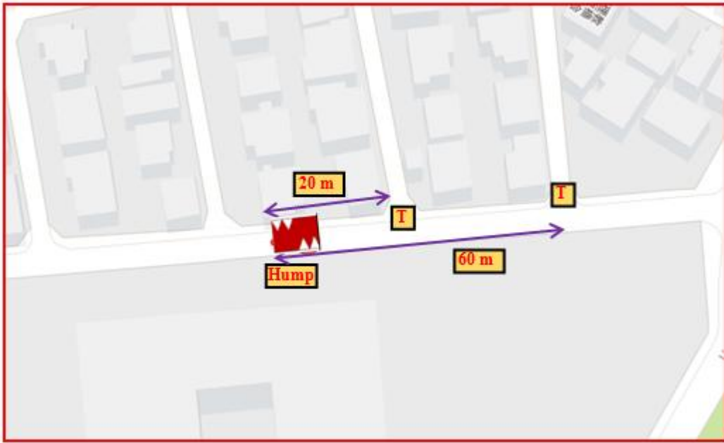
Fig. 2.10 Presence of T intersections at different distance from hump
