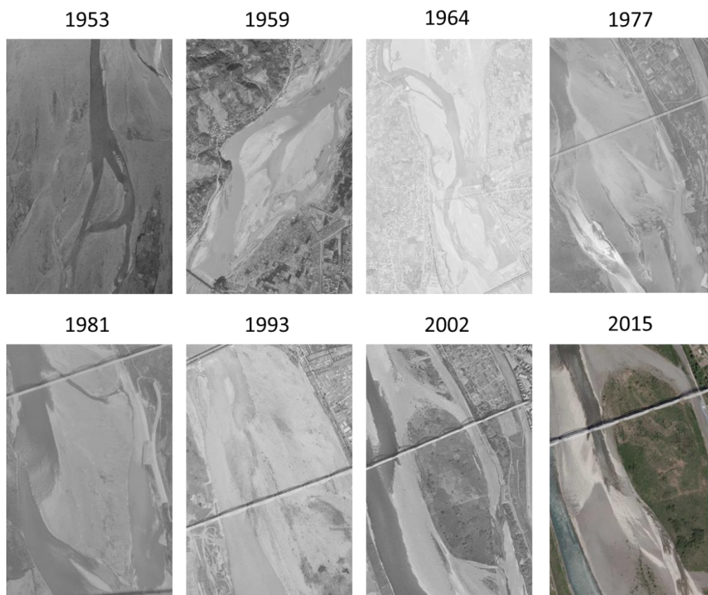
Figure 25. A representation of the chronosequential historical aerial imagery of the lower Fuji River showing its extended vegetation and sedimentary dynamics.
