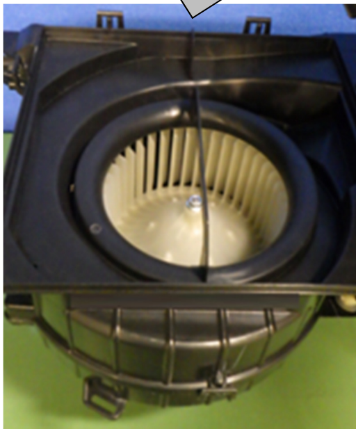
(B) Scroll casing and impeller
