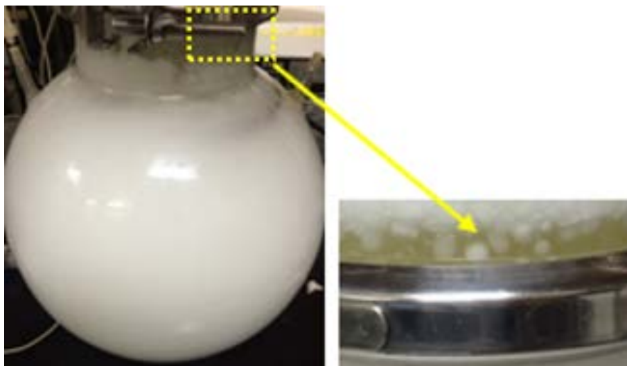
Fig. 5-10 Formation of the Emulsion phase at the water-oil interface at 10 °C ± 3 °C.
