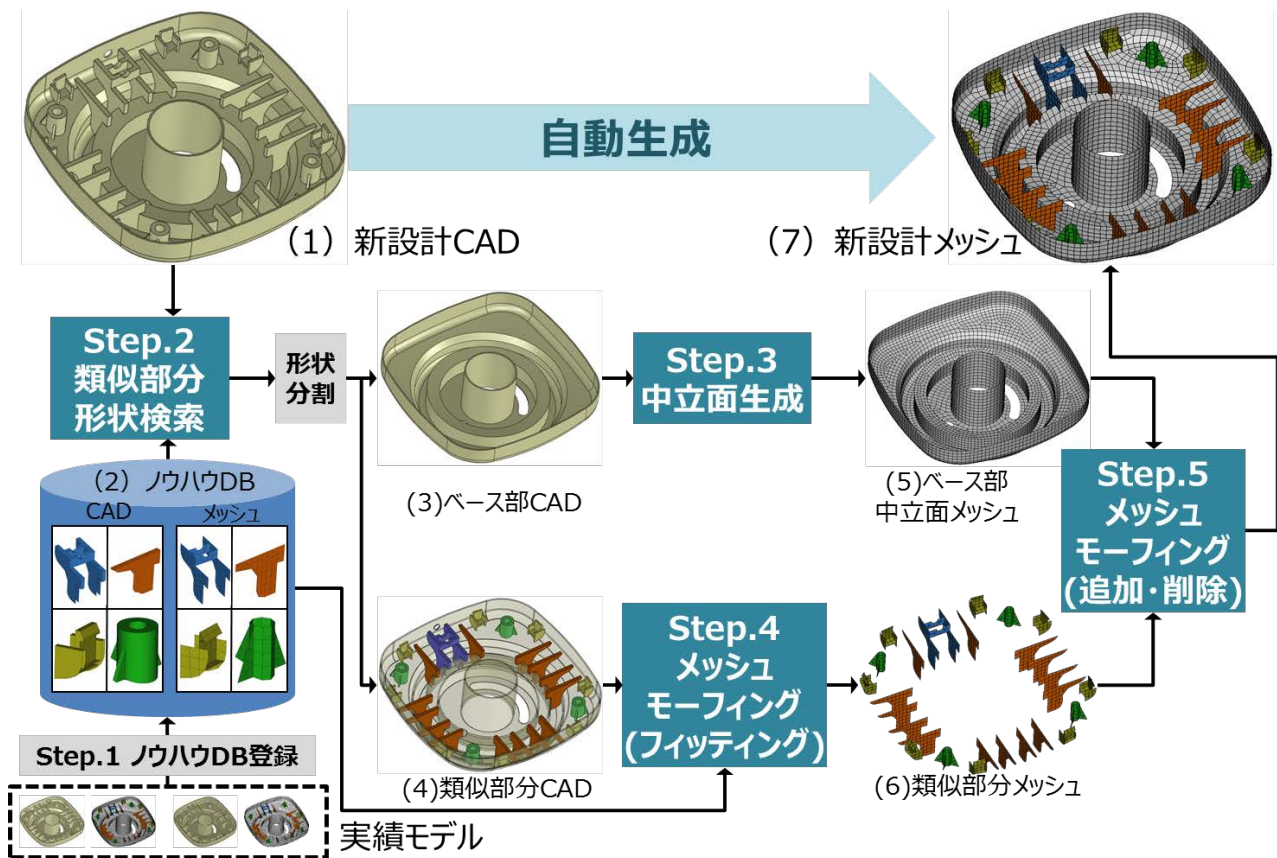
Fig. 2-1 High-precision analysis model generation technique for structures with complicated curved surfaces and protrusion shapes.
