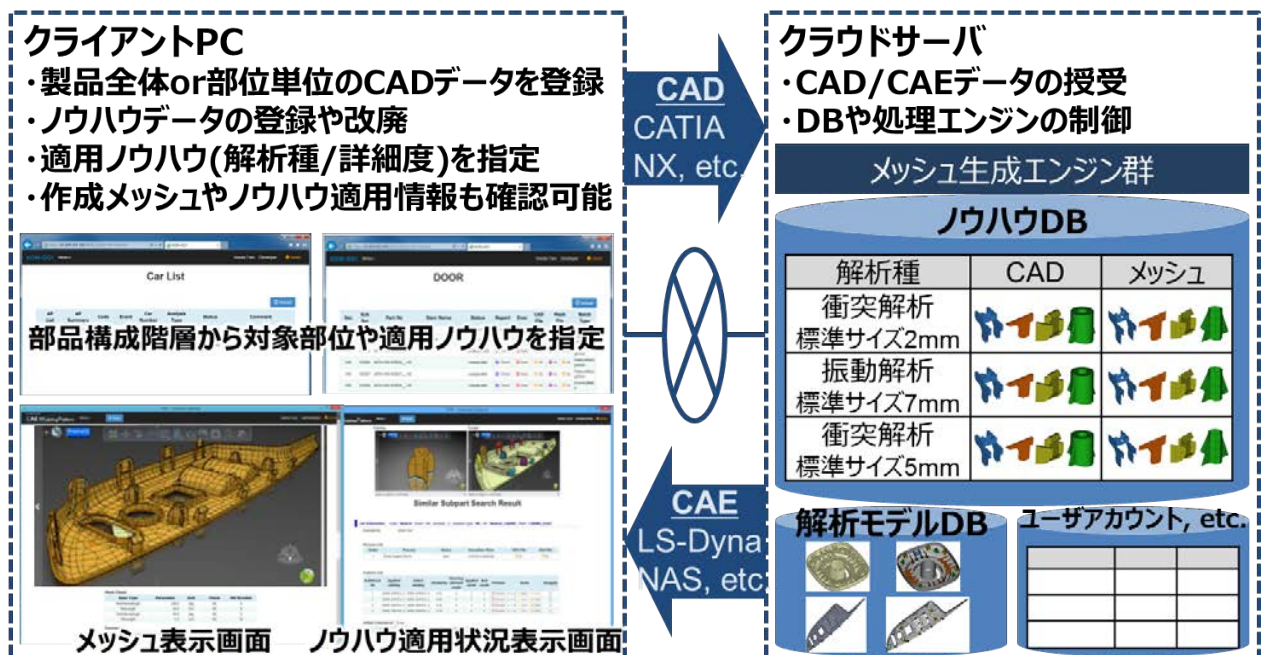
Fig. 3-1 Overview of system configuration.
