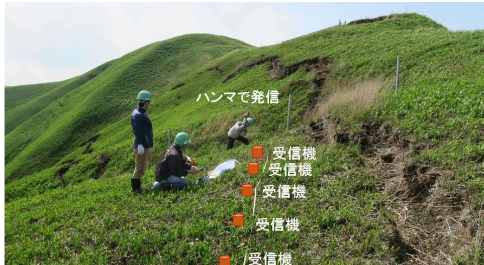
Figure 7.7 Seismic refraction test. Energy source a drop of hammer. The receivers are 8 geophones which set up with 1.5m of interval distance.
