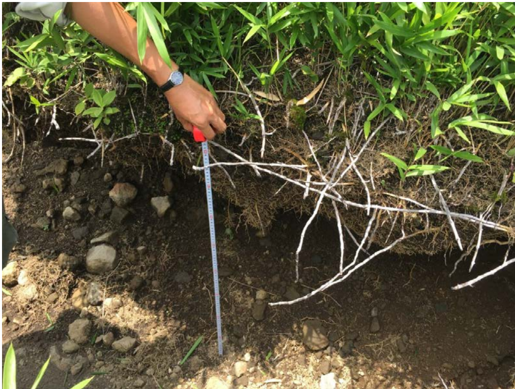
Figure 7.2 The depth of the crack is near 1m.
