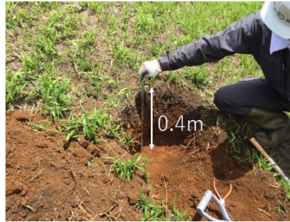
Figure 7.19 Undisturbed soil sample from a depth of 0.4m
