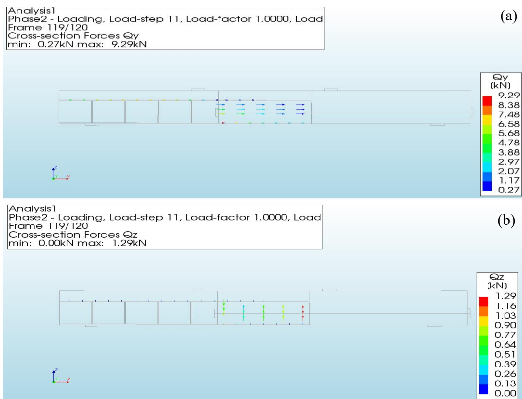
Figure 5. 36: Stud shear forces at 60kN design load; (a) horizontal and (b) vertical
