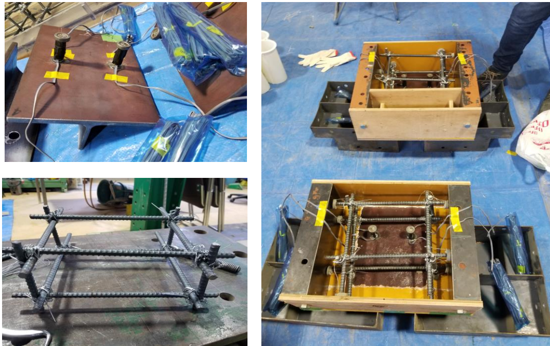
(a) Specimen assemble and formwork preparation
