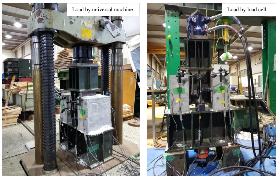
(b) Practical laboratory load setup for pushout specimen
