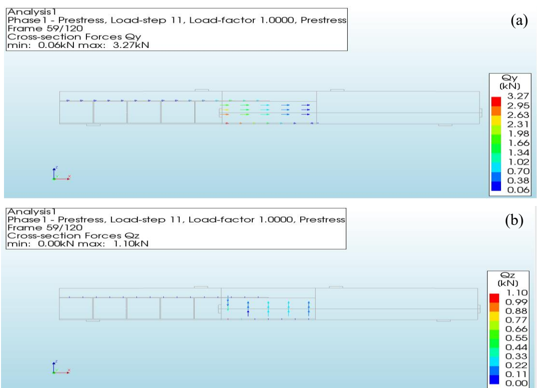
Figure 5. 35: Stud shear forces at prestressing phase; (a) horizontal and (b) vertical
