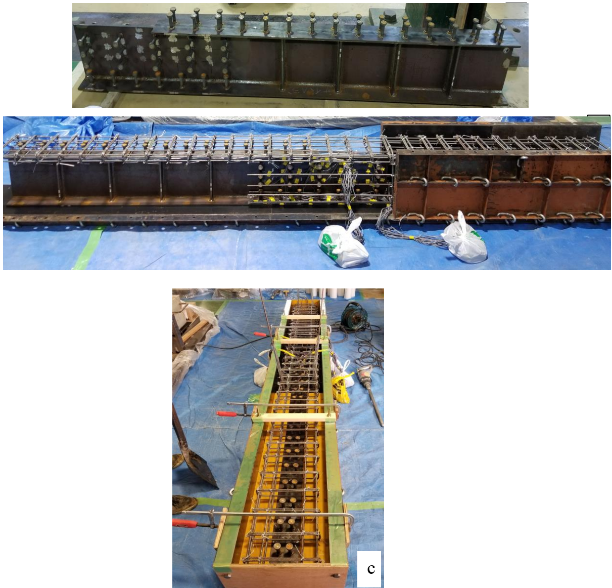
Figure 5. 4: Assembling of specimen. (a) steel girder with welded studs; (b) pasting of strain gauges and placement of rebars; (c) setting of formworks.
