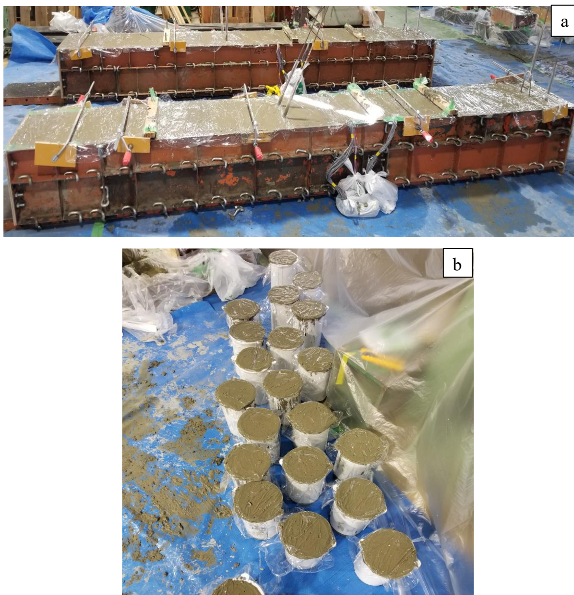
Figure 5. 5: Casting of specimen. (a) Hybrid girder; (b) Cylinder.
