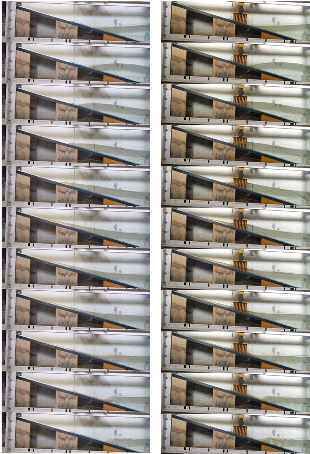
Figure 5-2 Photo snapshots of solitary wave runup on beach slope ( $s$ ) of  $1/4$ , wave height ( $H_o$ ) of 8.3cm and water depth ( $h_o$ ) of 22 cm.
