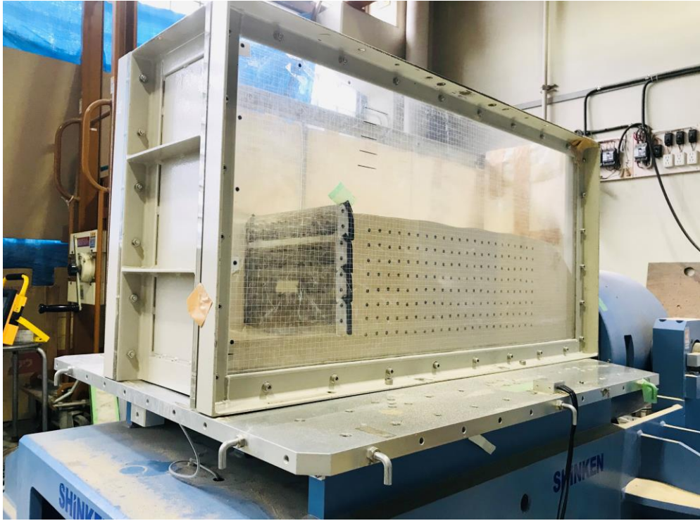
Figure 2 Shaking table facility
