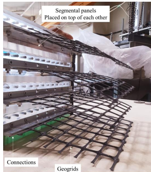
Figure 6(a) Reinforcement material for the MSE walls
