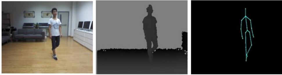
Figure 1.4: Sample images showing different modalities such as RGB, depth and skeleton in the RobotPKU RGBD-ID [7] dataset.
