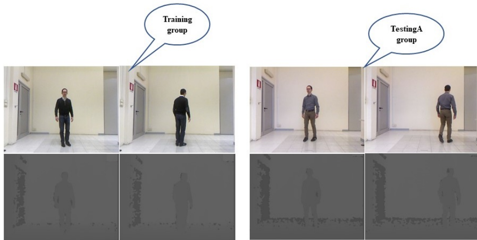
Figure 3.6: Example of the RGB and their corresponding depth images of the same person with different clothes.
