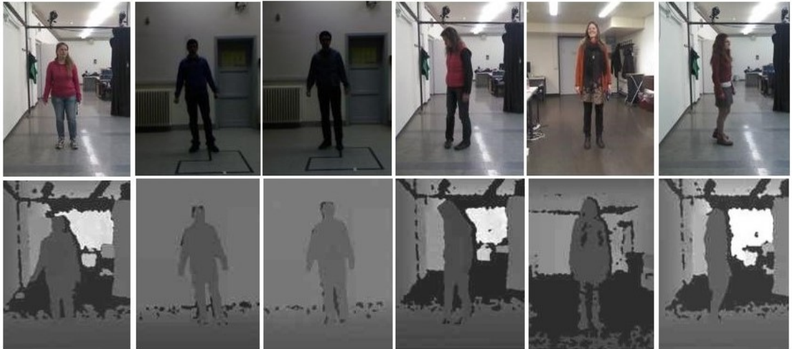
Figure 3.2: Examples of RGB and depth images captured in indoor environments. In Row 1, columns 1, 4, 5 and 6 show the RGB images in good illumination conditions, with columns 2 and 3 in poor illumination conditions accordingly. Row 2 shows the depth images of all RGB images.
