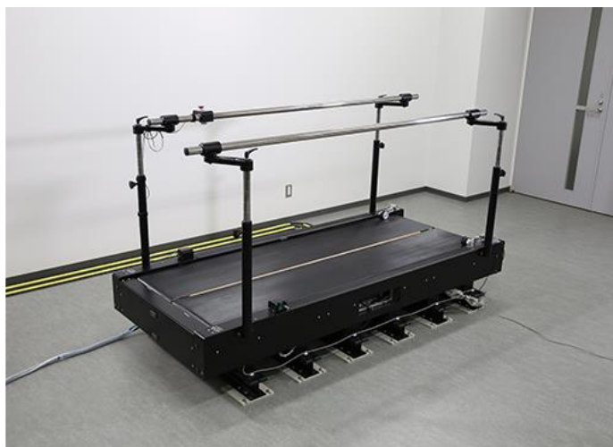
Fig.5.2 Treadmill with built-in force plate.
