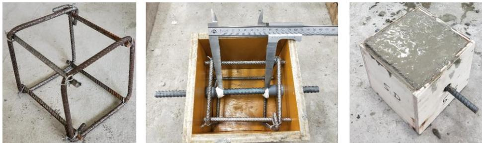
**Figure 5-2 Photographs of the specimen during casting**
