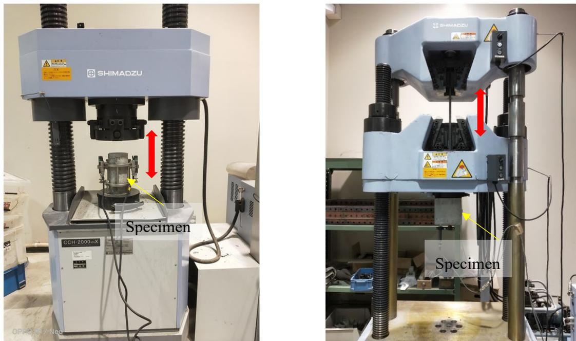
**Figure 5-7 Setup for (a) uniaxial compressive strength test and (b) pull out test in Universal Testing Machine (UTM)**
