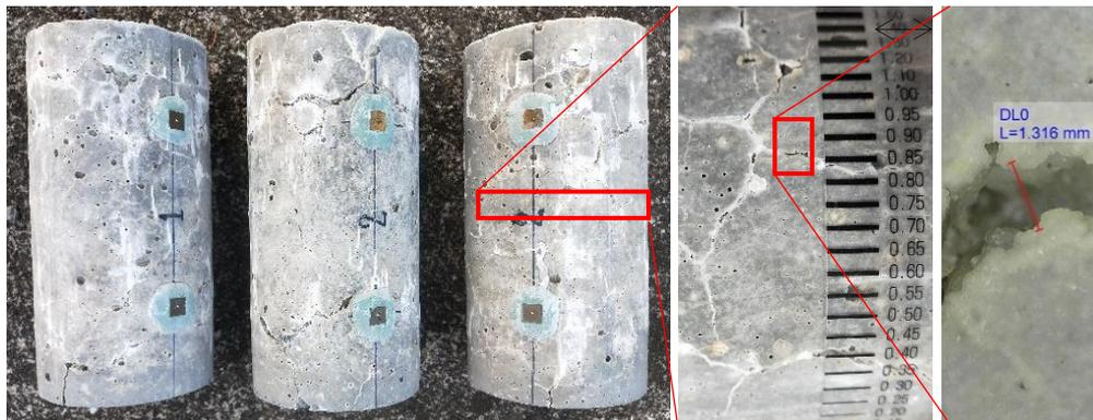
Figure 6-6 Condition of specimens before the mechanical test
