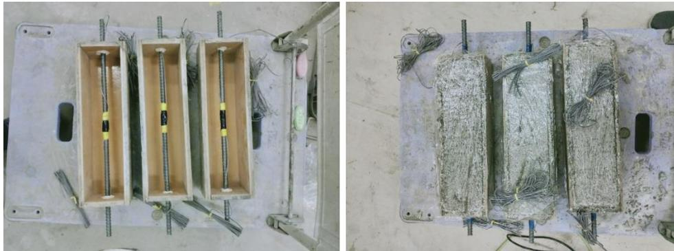
**Figure 3-2 Photographs of the specimens during casting**
