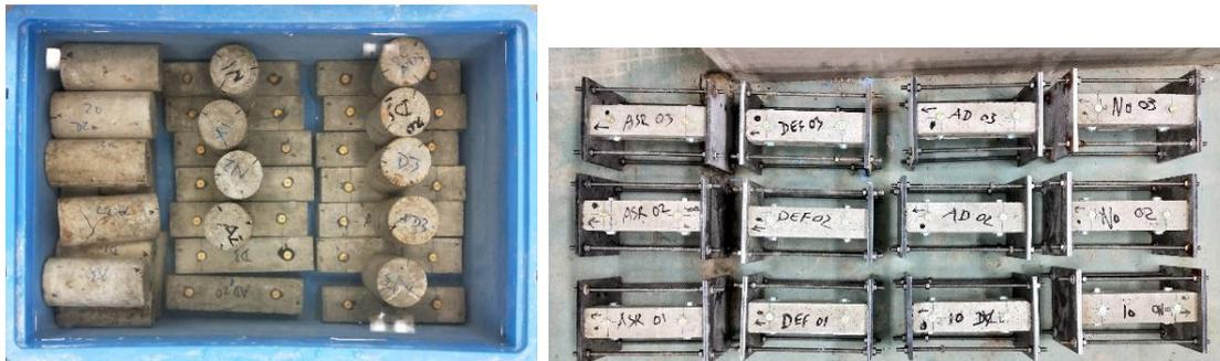
Figure 4-4 Specimens for (a) free and (b) restraint expansion
