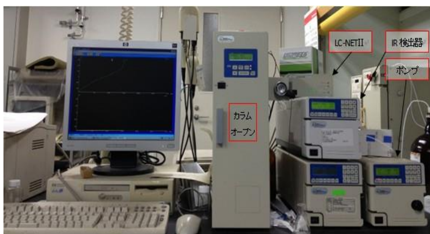
Figure 7. Experimental apparatus of GPC (HPLC Pump Jasco PU-2080; RI Detector Jasco RI-2031; Column Thermostat Jasco CO-2060).
