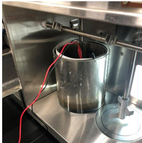
Figure 3.3b: Photo of the experimental setup for electrolytic treatment
