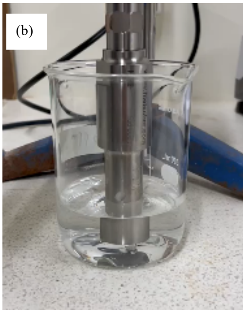
Figure 28. Dispersing soybean oil with an ultrasonic device. (a) UP400st (b)Before dispersing (c) After dispersing.
