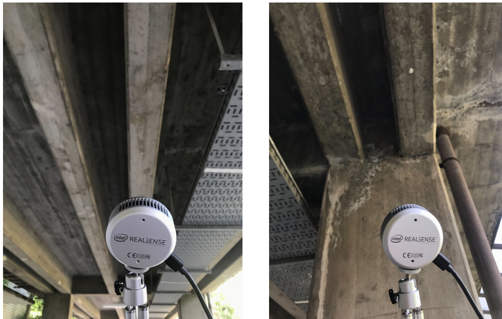
Fig. 83 Data Gathering using RealSense Lidar Camera L515
