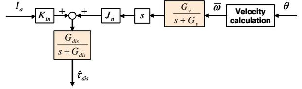
Fig. 3. Equivalent transformation form of disturbance observer
