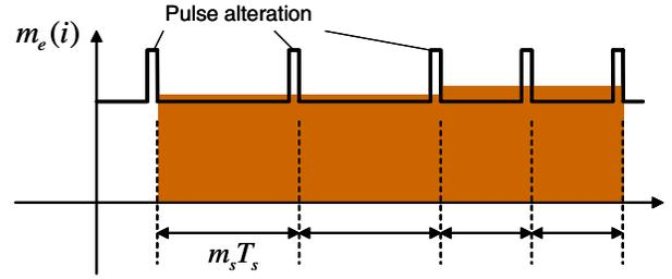
Fig. 5. Pulse number pattern in high-speed range
