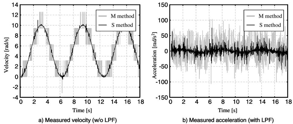
Fig. 8. Acceleration control with feedback derived by S method
