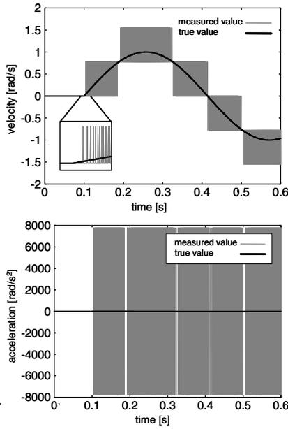
Fig. 4. Velocity and acceleration derived by finite-difference derivative
