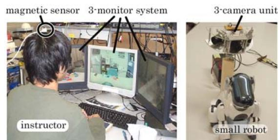
Fig. 2 System configuration of an instructor's site (left) and a robot's site (right)
