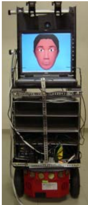
FIGURE 1- Prototype eye-contact robot.
