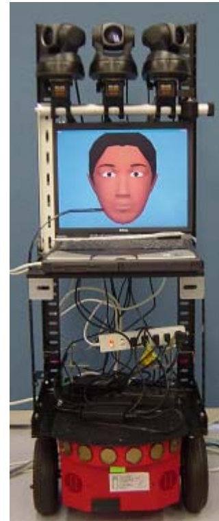
FIGURE 10- Robot with three cameras.
