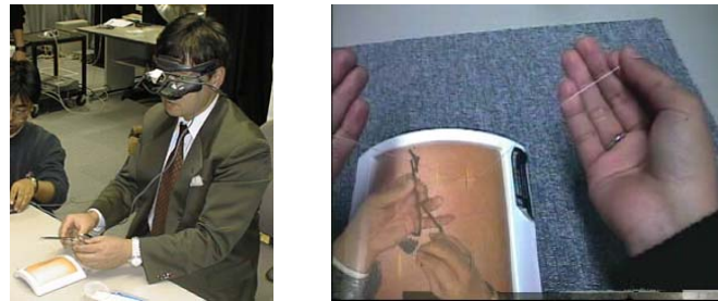
Fig 1. GestureView HMD being worn (left) Right: what is seen through the HMD – the remote instructor's gestures are superimposed on the other person's view taken by the cameras.
